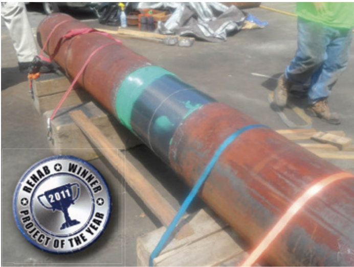
The simulated test of what the PipeMedic™ carbon laminate sleeve would look like once installed.
