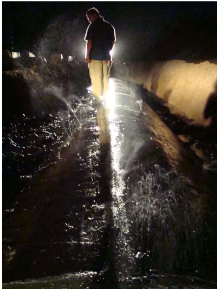
Fig. 2: After conventional crack sealing, the penstock failed to pass a second pressure test.
