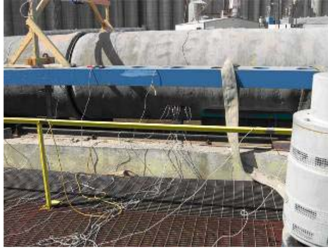
Figure 8: Strain Measurement Instrumentation Attached to Prototype
