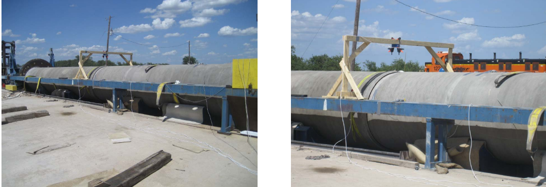
Figure 6a, b: Test Setup with Assembled Joint
