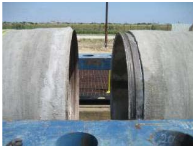
Figure 7: Swedged Bell and Spigot with a Rolled Groove Prior to Assembly
