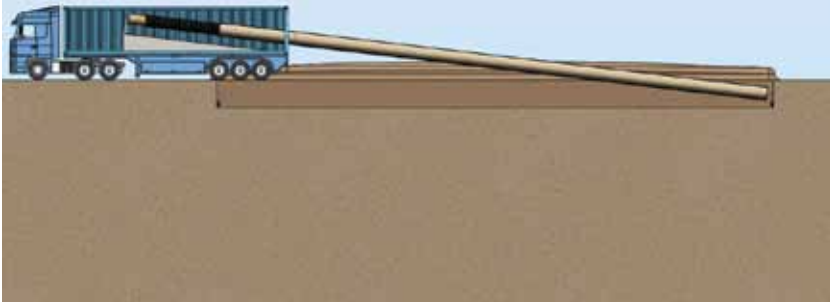
Conception of how Ehsani's mobile pipe-laying truck could create a pipeline of virtually infinite length Graphic illustration by Reynard Perrin and Joerg Schmit
