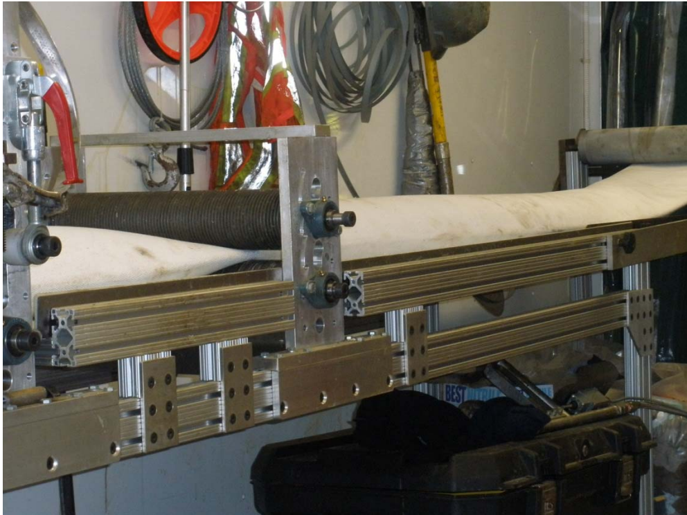
Figure 1: Tube filled with epoxy resin, roller system
