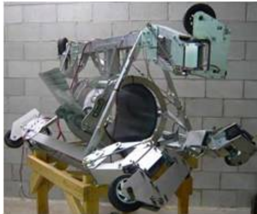
Fig. 9 – Robot for installation of PipeMedic™ laminates in pipes.
