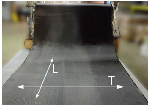
Fig. 1 – Biaxial carbon fabric with fibers oriented in both longitudinal (L) and transverse (T) directions.
