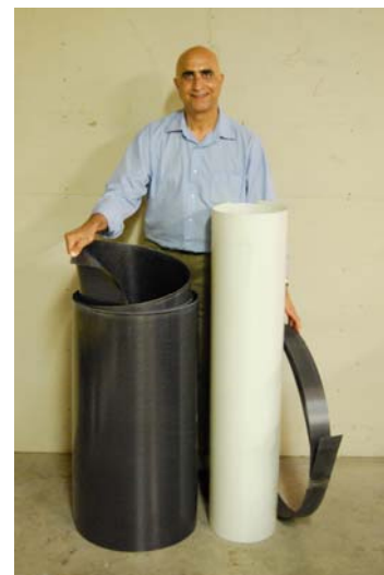
Fig. 4 - From left to right: flexible carbon and glass PipeMedic™ laminates
