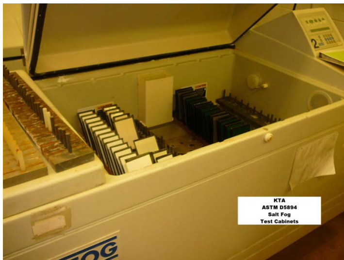
Figure 9 Test 7 Salt Fog Testing
