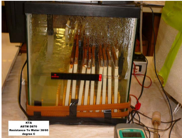
Figure 6 Test 1 Resistance to Water
