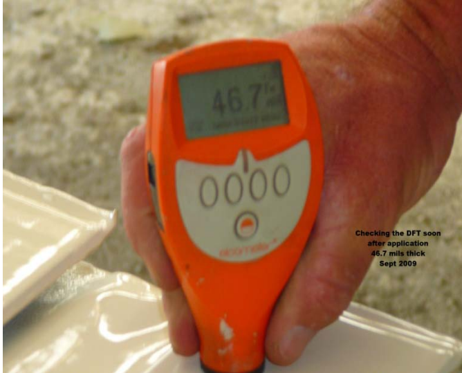
Figure 4 Dry Film Thickness Measurement
