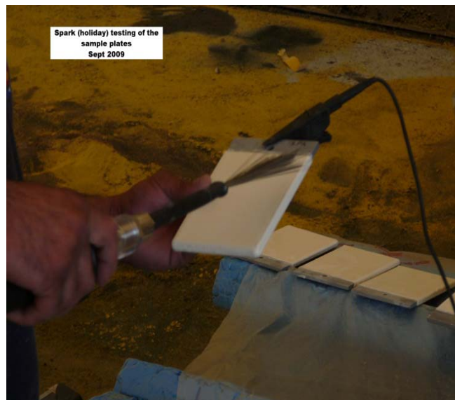
Figure 5 Holiday Testing of Coated Sample Plates
