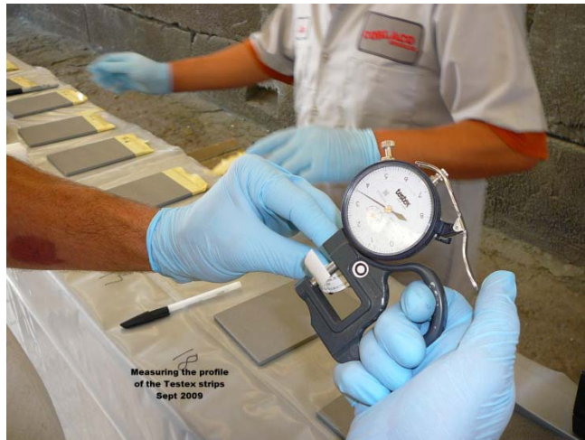
Figure 1 – Replica Tape Testing
