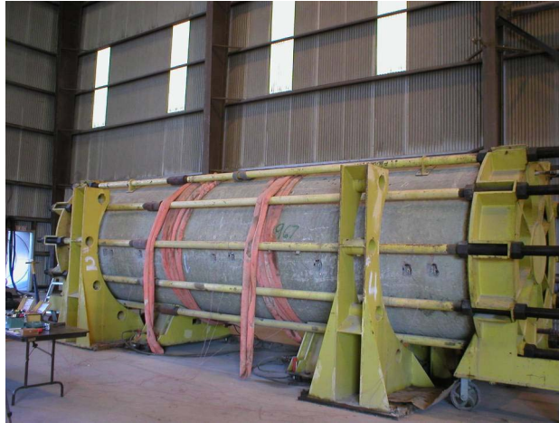
Figure 1. Hydrostatic testing of PCCP with broken prestressing wires.
