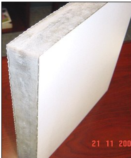
Figure 1: Cross-section of GRP laminate.
