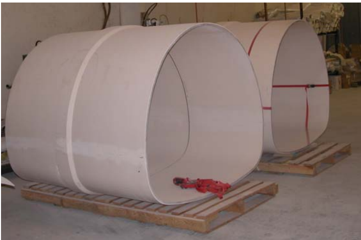
Figure 4: Non-circular slipline pipes
