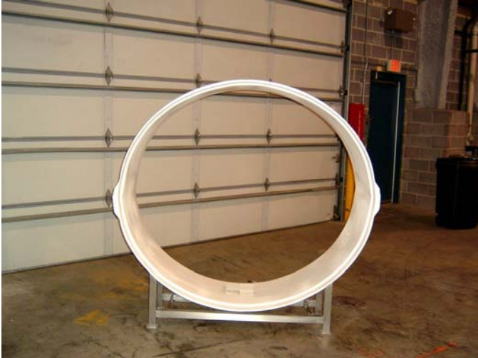
Figure 2: GRP segment (2 panels) used in Fort Wayne.
