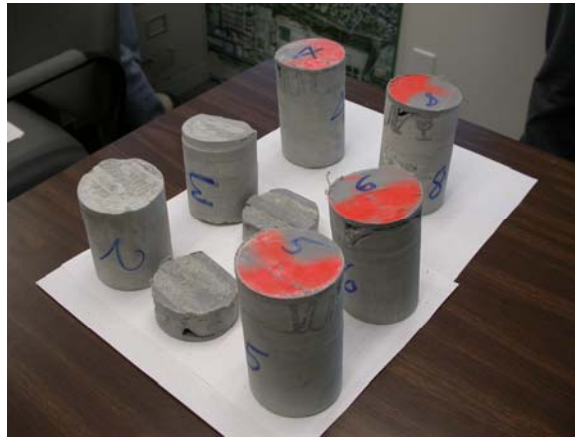
Figure 9. Grout Penetration Core Samples
