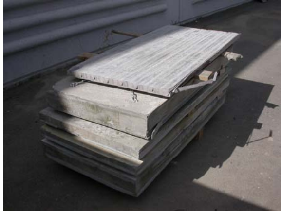
Figure 7. Cast box samples prior to cutting beams
