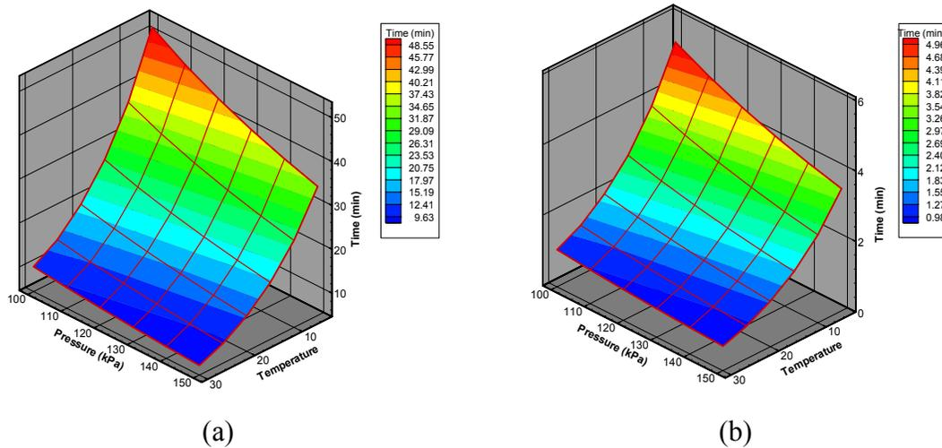
**Figure 9.** Resin Flow Analysis of the Reinforcing Experiment: (a) Satin Woven Preform; (b) Stacked Preform.
