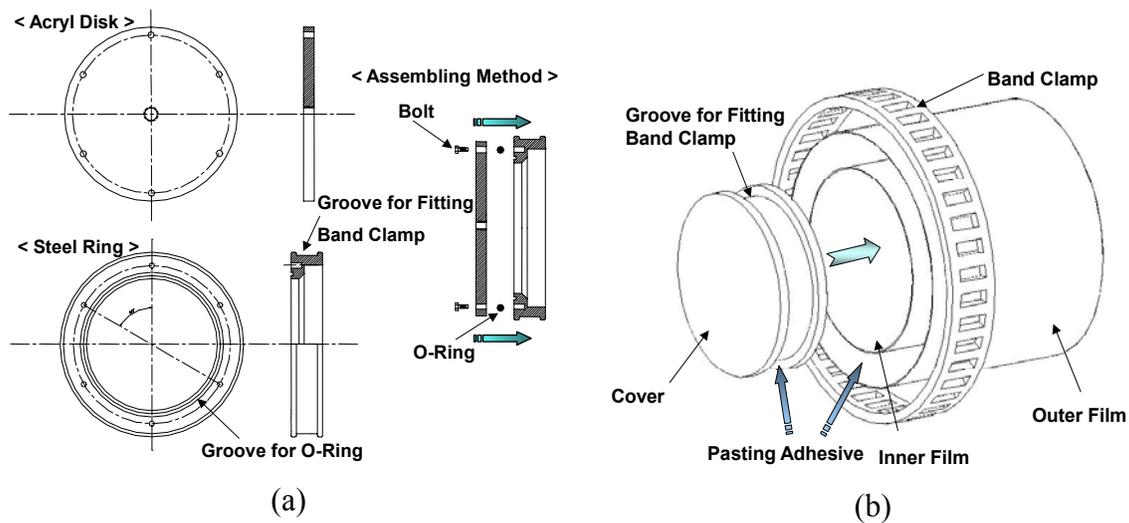
**Figure 3.** Cover Design and Assembling Method: (a) Detailed Design of the Cover (Steel Ring + Acryl Disk) and Its Assembling Method; (b) Clamping Method of Covers and Positions for Pasting Adhesive.
