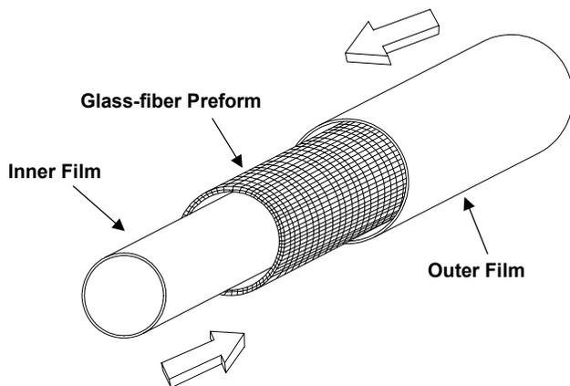
**Figure 2.** Preparation of the Reinforcement.
