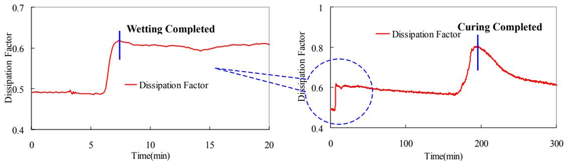
**Figure 8.** Dissipation Factor of Unsaturated Polyester during the Repairing Process Measured by Dielectrometry.
