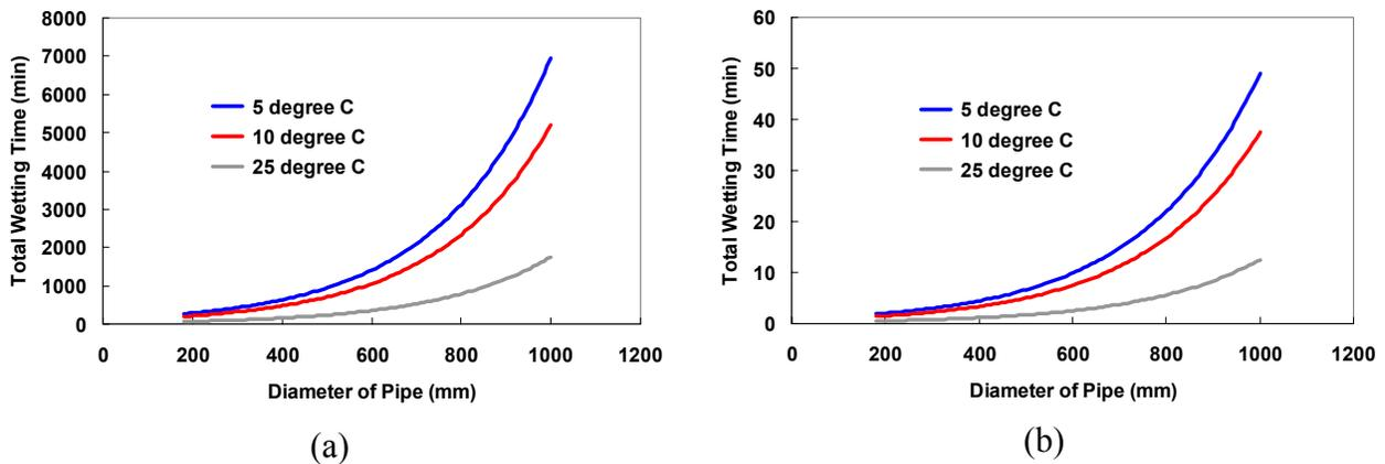
**Figure 6.** Resin Flow Analysis and Predictions of Wetting Time w.r.t. the Temperature and Diameter of Pipes: (a) Satin Woven Preform; (b) Stacked Preform.
