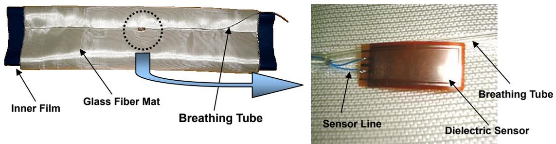
**Figure 7.** Reinforcement with a Breathing Tube and a Dielectric Sensor whose Dimension Is  $9 \text{ mm} \times 250 \text{ mm} \times 168 \text{ }\mu\text{m}$ .
