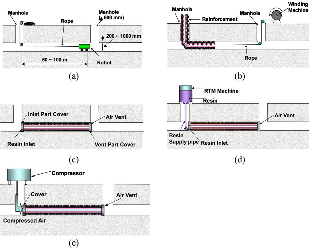
**Figure 1.** Repairing-reinforcing Processes of Underground Pipes with RTM: (a) Removing Deposits and Protrusions in the Pipe; (b) the Reinforcement Is Connected to a Rope and Pulled; (c) Closing Two Covers at the both Ends of Reinforcement; (d) Resin Injection; (e) Resin Wetting and Curing.
