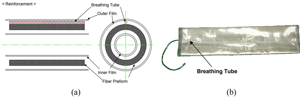
**Figure 5.** Void Removal Method Using the Porous Breathing Tube: (a) Schematic Diagram; (b) Photograph of the Reinforcement Applying This Method.
