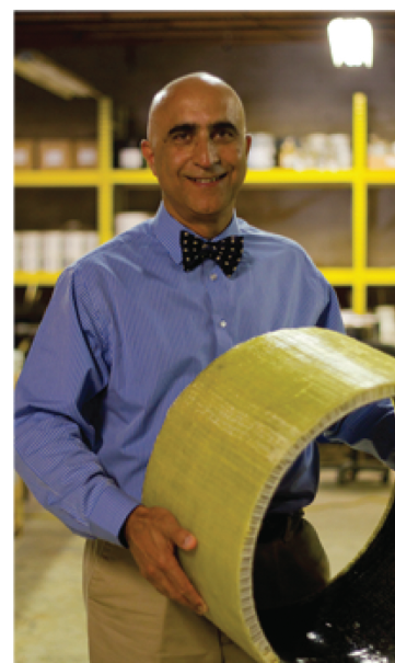
Professor Ehsani holding a section of InfinitPipe™, a revolutionary on-site manufactured carbon FRP and honeycomb pipe that can be built to any length and diameter, eliminating leaking joints and transportation costs.
