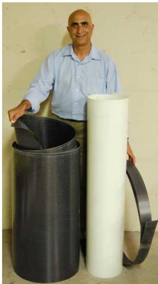
Figure 1: From left to right: carbon and glass super laminates; carbon laminate strip.
