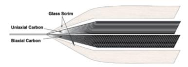
Fig. 1: Super laminates can be constructed with multiple layers of unidirectional or biaxial fabrics
