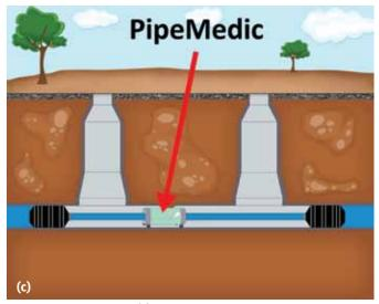
Fig. 4: Repair of pipes: (a) conventional method requiring above ground bypass; and (b) and (c) using super laminates with bypass through the pipe
