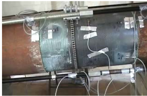
Figure 4. Instrumented laminate during test.
