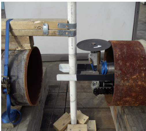
Figure 14. Simulated drip pot with standpipe laboratory test set-up.
