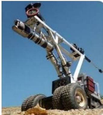
Figure 1. Multi-sensor inspection device (crawler type).
