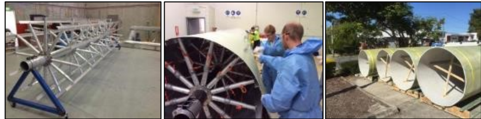
Fig. 3. Construction of StifPipe® at QuakeWrap facilities in Brisbane, Australia
