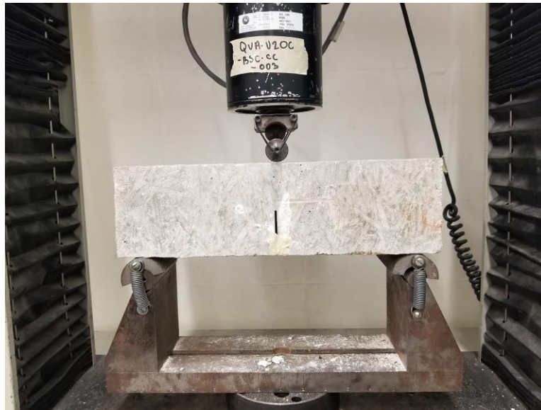
Figure 11.2 – Shear bond test set-up
