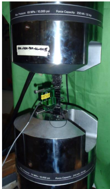
Figure 5.1 - Tensile test set-up
