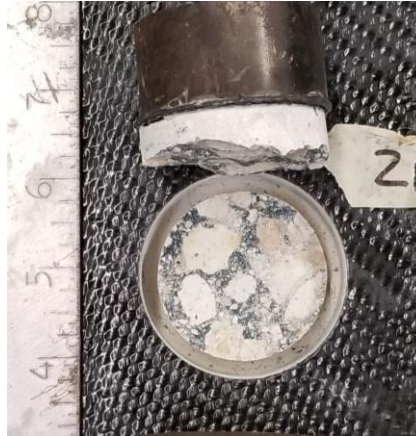
Figure 10.3 - Typical failure of performed tension bond strength test.
