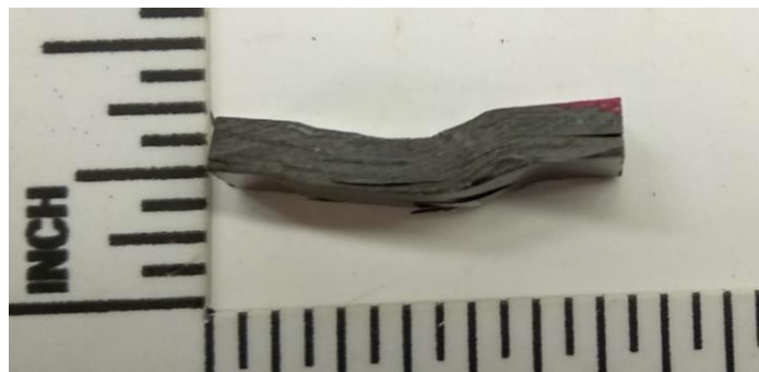
Figure 9.2 – Representative type 1 failure mode showing interlaminar shear between plies
