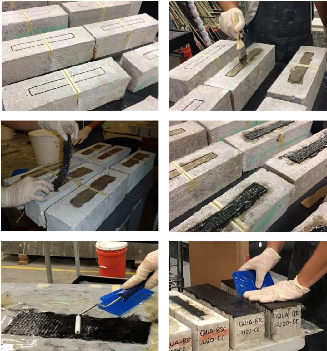
Figure 4.2 – FRP system installation on concrete substrate
