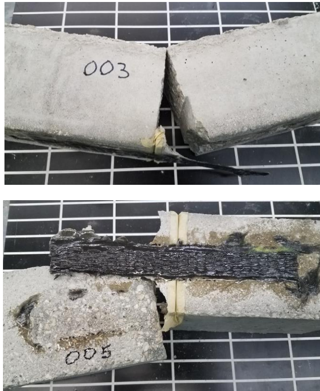
(b) Figure 11.3 – (a) Possible failure mode types for shear bond test; and (b) representative shear bond failure mode (side and plan views)
