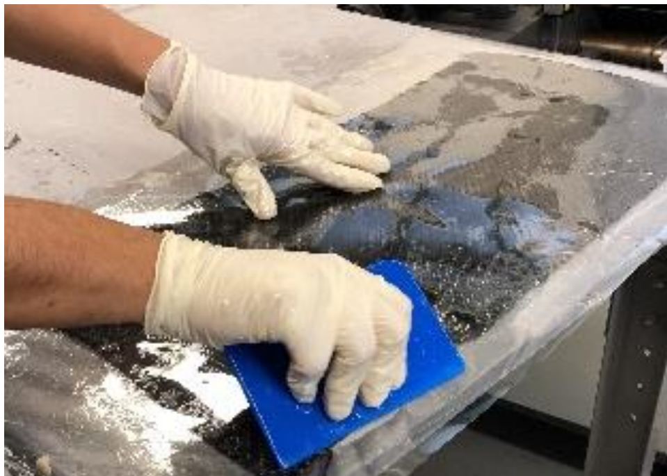
Figure 4.1 – Preparation of FRP panels by manual wet layup process
